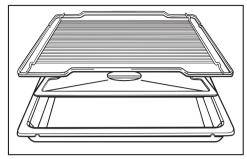
The anti-splash tray should be placed in the deep-sided grill pan when grilling or roasting. The juices from the food being cooked collect under the anti-splash tray. This prevents them from spitting and making the oven dirty. The juices can then be used for making gravy and sauces.
